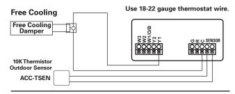
Free Cooling utilizes the Y1 terminal for the operation of 1st stage cooling. If mechanical (compressor) cooling is also present, the mechanical cooling is connected to the Y2 terminal in this instance.
