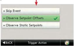
In the above example; if the price threshold is exceeded, the thermostat will invoke the 'Offset Setpoints' configured for an ADR event until the event is over.
